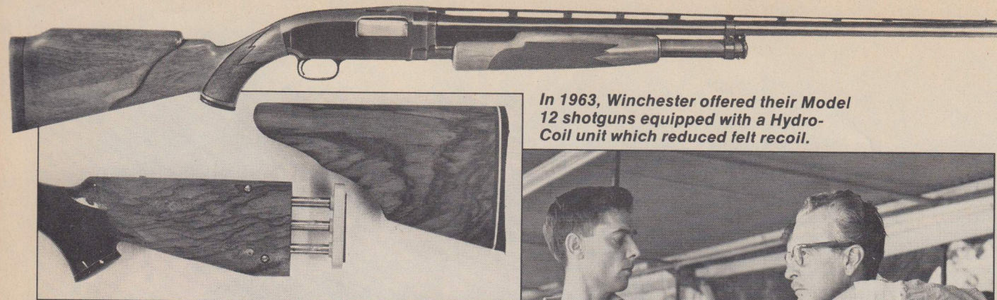
The Hydro-Coil acts like a shock absorber as the gunstock's comb remains stationary while the rest recoiled rearward within the comb.
