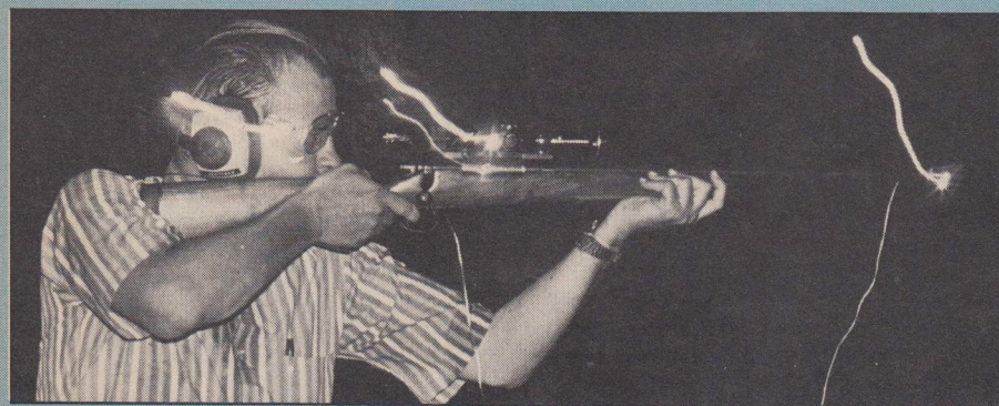
Surprisingly, this 7 mm Remington Magnum with factory 175-grain ammunition churned up less recoil than the .30-06 Springfield with handloads used in these tests—only 19.3 foot pounds of free recoil energy in a rifle weighing 8¾ pounds. The milder recoil is verified by trace measurements—only 7.6 inches vertical muzzle rise, while the shooter's head was displaced by only 5.8 inches. Certainly, maximum handloads would develop more velocity and more recoil, but these results are interesting in view of the overall effectiveness of this magnum cartridge on game animals.
