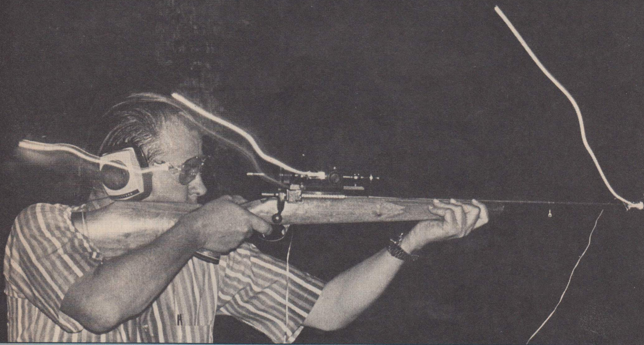
Results of a harder kick than most American hunters have ever felt are dramatically illustrated here. The rifle is chambered for the .416 Taylor wildcat cartridge and weighs 9½ pounds. The 400-grain bullet, being driven better than 2,400 feet per second, generates 44.5 foot pounds of free recoil energy. The total rearward rifle movement is 13½ inches and vertical muzzle rise equals 14½ inches. The shooter's head was driven not quite one foot to the rear, but the upward movement of the comb against the rifleman's cheek in this well-stocked rifle is less than 1½ inches. Very close examination of the trace of the bulb on the author's shooting glasses reveals an initial "whiplash" of his head forward as recoil drives his shoulder rearward.
