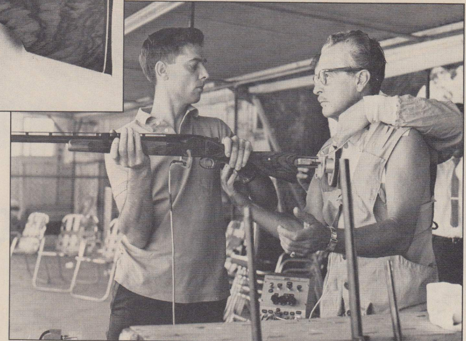
Recoil can play havoc on a shooter's pulmonary and nervous systems. Here a shooter was "wired" to an oscilloscope to measure the devastating effects of recoil on the human body.
