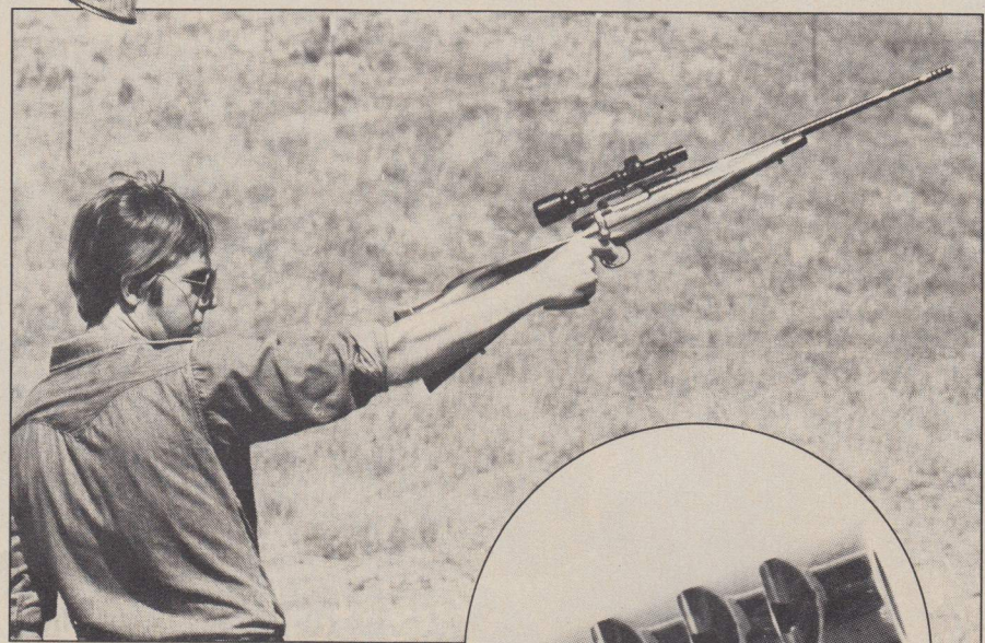
Thanks to a thumbhole stock design and muzzle brake, rifles in the .30 caliber class can be used one-handed. The shooter absorbs most of the recoil in his hand and arm, while the muzzle brake (inset) redirects gasses to keep muzzle jump and recoil down to a tolerable level.
