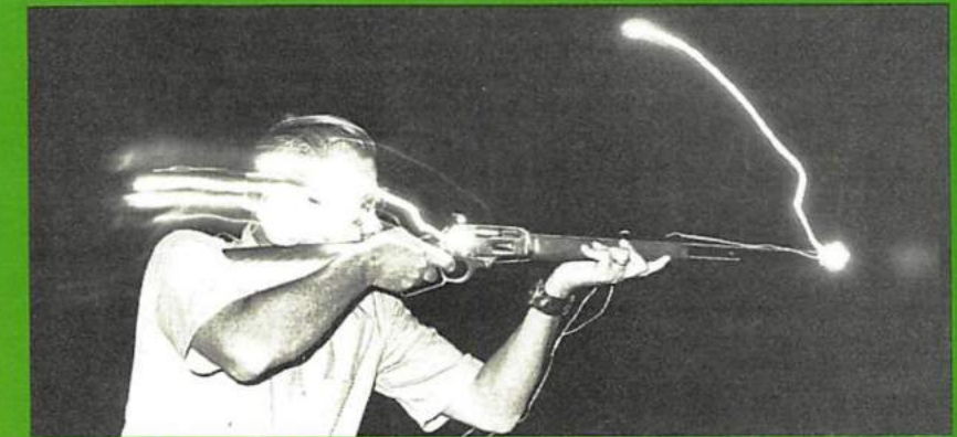
New Marlin M1895 .45-70 (7¼ lbs.), boosting a 400-grain bullet at 1665 fps, delivers nearly as much free recoil energy as a normal .375: 38.8 ft./lbs. Wavy line traced by light on Wootters' glasses shows how his head rocked under impact.
