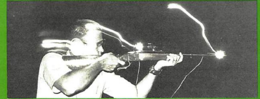
Ruger No. 1 .45-70 (8½ lbs.), heaving a 500-grain slug at 1775 fps, clobbers the shooter with 38.7 ft./lbs. recoil, much more than the .30-06 with 180-grain bullets.
