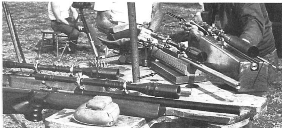
Bolt handle is lengthened because of massive stock (upper arrow) on a 1000-yard benchrest rifle. Rifle bolted to lead block (lower arrow) weighs over 150 lbs.
