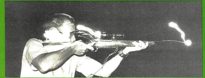
A 152-grain bullet, moving at 2825 fps at the muzzle, churning up only 13.5 ft./lbs. in recoil energy, set the eight-lb. Ruger M77 .308 back less than seven inches.
